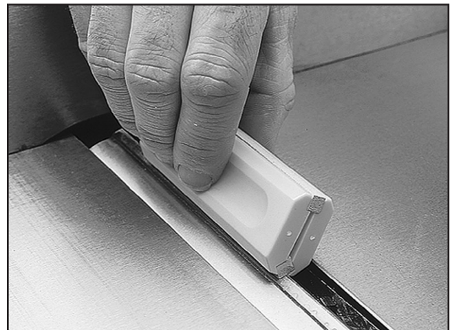
Figure 37. G3631 Jointer/Planer Knife Hone.
